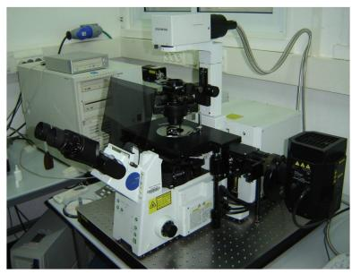
This inverted LSCM is housed in microscopy unit room (112) in Plant Science (Fruit Tree building) institute. It has three PMT and one transmitted light detectors. It is equipped with the following:
